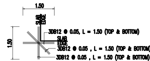
TYPICAL REINFORCEMENT AT CORNER
